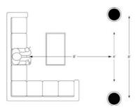
Figure 1. Typical placement for stereo listening.
